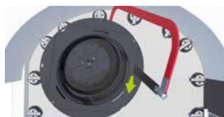
9. Cut one side of the pedestal.
