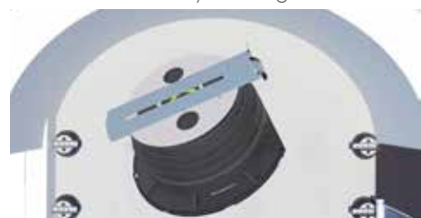
7. Place the SUPACLPP perpendicular to the wall.
