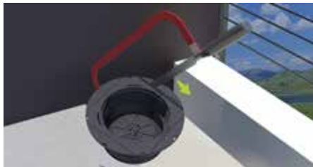
1. Cut one side of the pedestal.
